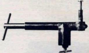
perfectly as fast as fifteen to twentyfive per minute, according to skill; rightly used, it just fills the grooves and no more, leaving the bands bare. This is essential for fine work, for if there be more grease on one side of bullet than on the other, it displaces that bulk of lead on upset, throwing the bullet out of balance. If the mould is round, as mine are, no wiping of bullet is necessary. Dies are made
