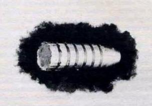
bullet back; the result is an uneven, wobbling flight. The greatest essential for perfect shooting is to deliver the bullet perfectly from the muzzle; that being done, atmospheric conditions and gravity alone govern its flight; the result is accurate shooting. To so deliver the bullet, it must have a perfect base, and be perfectly centred, and have uniform velocity.
