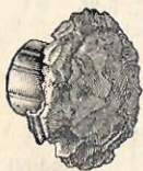
The Way a .401 Caliber Soft Point Bullet Mushrooms. Side View. Actual Size.
